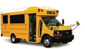
With an optional flat-floor, this 30-passenger school bus provides unmatched versatility, while its signature aerodynamic design helps increase this dual-wheel's fuel efficiency. Wheelchair package shown with optional flat floor and raised roofline.
